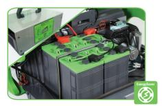
Extremely large battery compartment. Available with non maintenance Gel type **Power Battery** batteries and **BLS** standalone charger that includes **TCL** technology, allowing best recharge management of batteries that can double battery life time.
