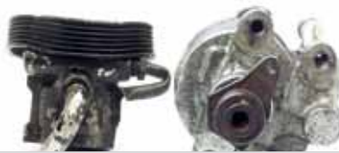
Pulley is damaged and hub broken
