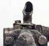
Bend or broken connections
